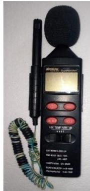
**Gambar 3.** *Environment Meter* Krisbow KW06-291
