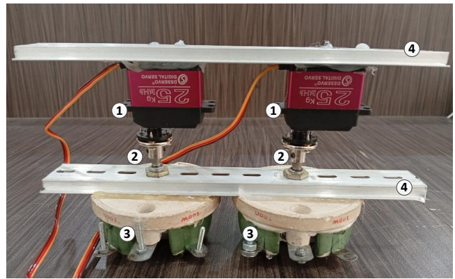
Figure 6. Proposed servo-controlled variable resistor (1) servo (2) mechanical coupling (3) 100 ohm 100 W rheostat (4) mounting
